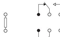
Note: JW 2 Form A is as shown in the diagram above except the N.C. terminals are not present.
