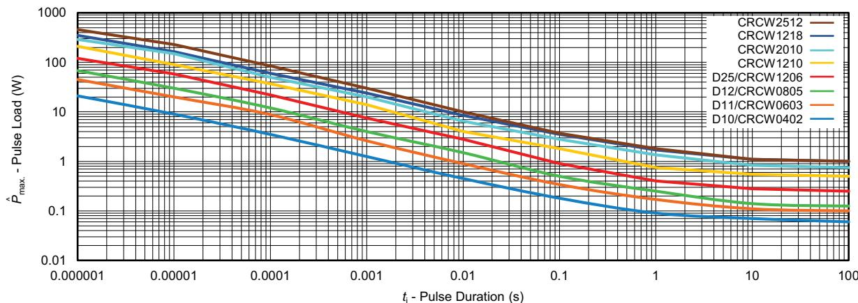
Maximum pulse load, single pulse; applicable if  $\bar{P} \rightarrow 0$  and  $n < 1000$  and  $\hat{U} = \hat{U}_{\max.}$ ; standard operation mode, for permissible resistance change equivalent to 8000 h operation
