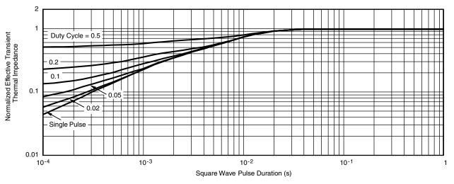
Normalized Thermal Transient Impedance, Junction-to-Case
