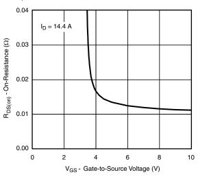
On-Resistance vs. Gate-to-Source Voltage
