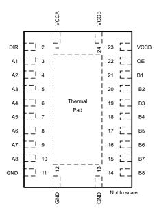
Figure 5-2. RHL Package, 24-Pin VQFN (Top View)
