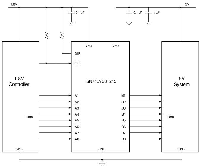
Figure 9-1. Typical Application Circuit
