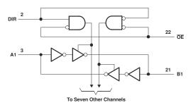
Logic Diagram (Positive Logic)
