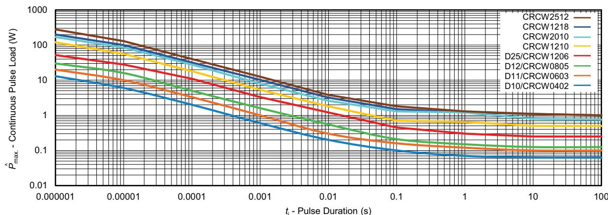
Maximum pulse load, continuous pulses; applicable if  $\bar{P} \leq P(v_{\text{amb}})$  and  $\hat{U} = \hat{U}_{\max.}$  for permissible resistance change equivalent to 8000 h operation
