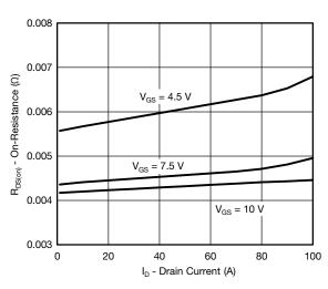
On-Resistance vs. Drain Current
