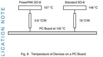
Fig. 8 Temperature of Devices on a PC Board
