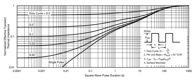
Normalized Thermal Transient Impedance, Junction-to-Ambient
