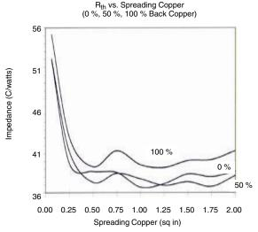
Fig. 6 Spreading Copper Junction-to-Ambient Performance
