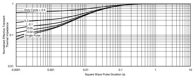
Normalized Thermal Transient Impedance, Junction-to-Case
