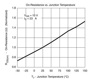
Fig. 7 MOSFET R<sub>DS(on)</sub> vs. Temperature
