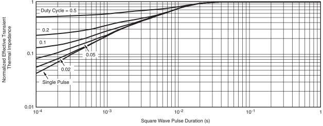
Normalized Thermal Transient Impedance, Junction-to-Case
