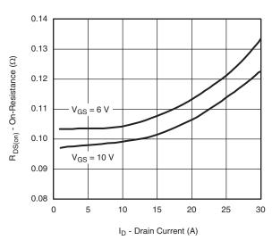
On-Resistance vs. Drain Current and Gate Voltage
