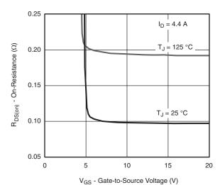
On-Resistance vs. Gate-to-Source Voltage
