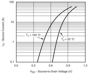
Source-Drain Diode Forward Voltage
