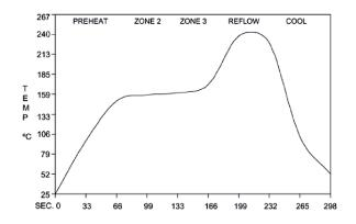
Fig. 3 Solder Reflow Temperature Profile
