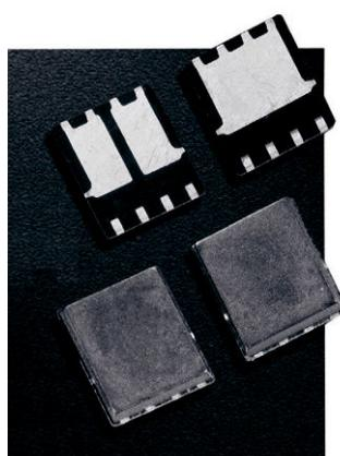
Fig. 1 PowerPAK 1212 Devices
