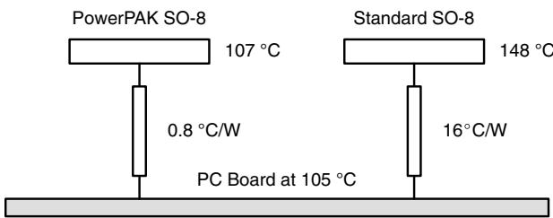
Fig. 8 Temperature of Devices on a PC Board
