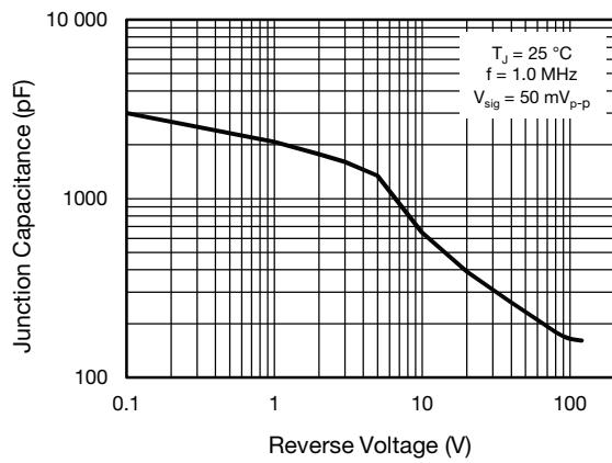
Fig. 5 - Typical Junction Capacitance Per Diode
