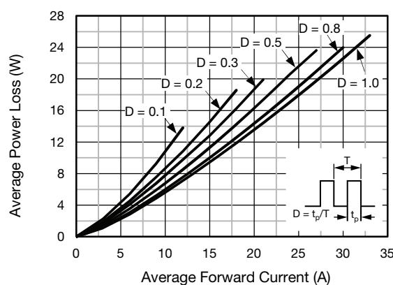
Fig. 2 - Forward Power Loss Characteristics Per Diode
