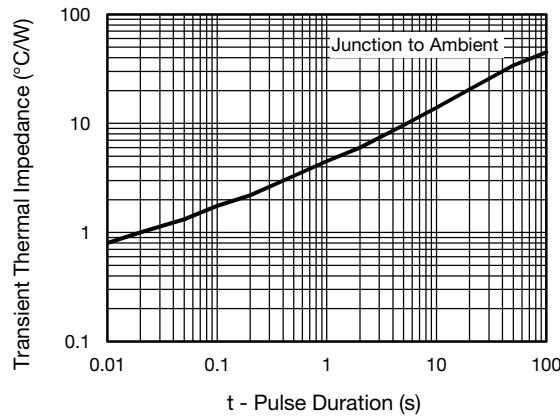
Fig. 6 - Typical Transient Thermal Impedance Per Device
