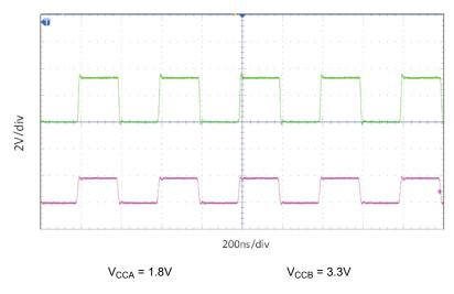
Figure 8-2. Level-Translation of a 2.5MHz Signal
