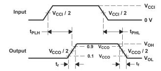
Figure 6-5. Propagation Delay Times
