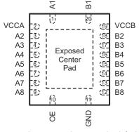
The exposed center pad, if used, must be connected as a secondary ground or left electrically open.
