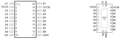
Figure 4-3. PW or DGS Package, 20-Pin TSSOP or Figure 4-4. RKS Package, 20-Pin VQFN (Top View) 20-Pin VSSOP (Top View),
