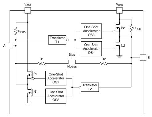
Figure 7-1. Architecture of a TXS0108E Cell
