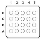
Figure 4-1. ZXY Package, 20 BUMP (Bottom View)
