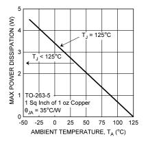
Figure 28. Maximum Power Dissipation vs Ambient Temperature for DDPAK/TO-263 Package
