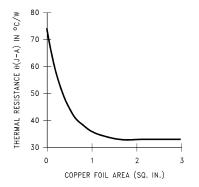
Figure 27.  $\theta_{JA}$  vs Copper (1 Ounce) Area for the DDPAK/TO-263 package
