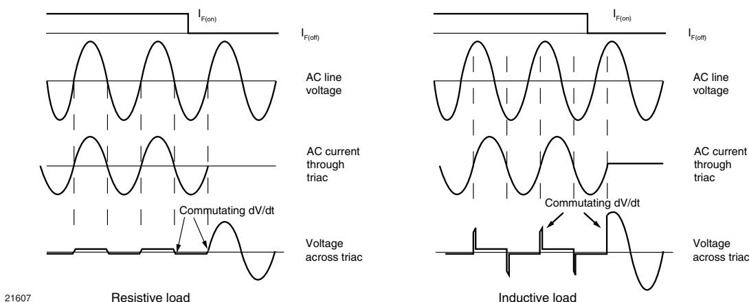
Fig. 8 - Waveforms of Resistive and Inductive Loads
