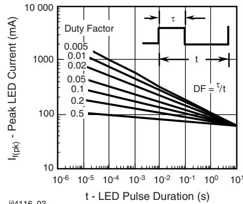
Fig. 3 - Peak LED Current vs. Duty Factor,  $\tau$
