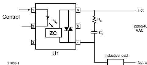
Fig. 11 - Basic Direct Load Driving Circuit
