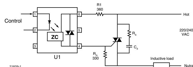
Fig. 12 - Basic Power Triac Driver Circuit
