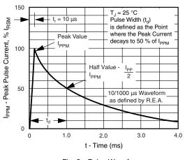
Fig. 3 - Pulse Waveform
