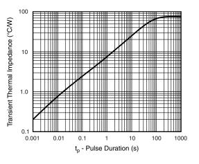
Fig. 5 - Typical Transient Thermal Impedance
