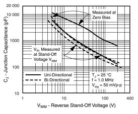
Fig. 4 - Typical Junction Capacitance Uni-Directional
