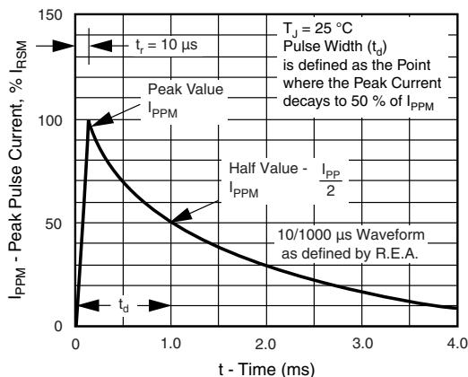
**Fig. 3 - Pulse Waveform**
