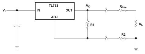
Figure 22. Regulator With Current-Set Resistor
