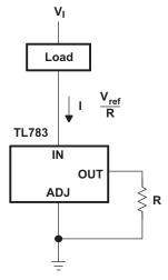
Figure 16. Current-Sinking Regulator
