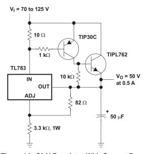
Figure 14. 50-V Regulator With Current Boost
