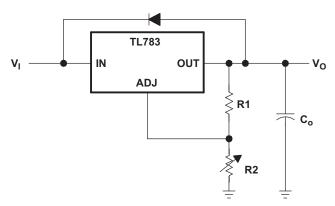
Figure 21. Regulator With Protective Diode
