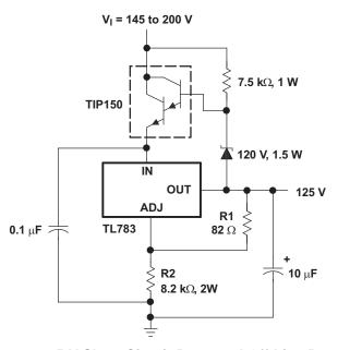
Figure 13. 125-V Short-Circuit-Protected Off-Line Regulator
