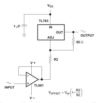
Figure 18. High-Voltage Unity-Gain Offset Amplifier
