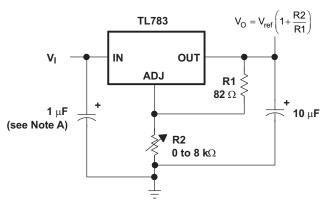
A. Needed if device is more than 4 inches from filter capacitor
