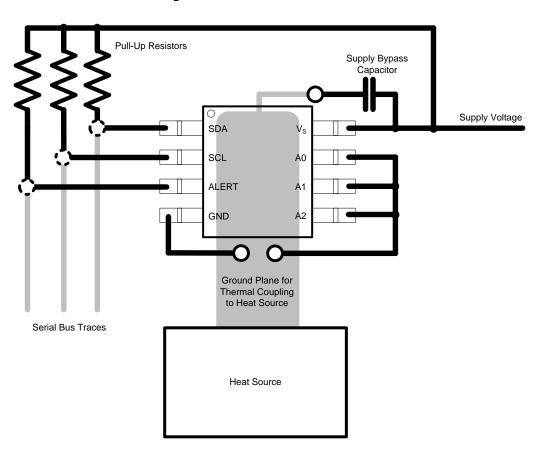
Figure 20. TMP275 Layout Example
