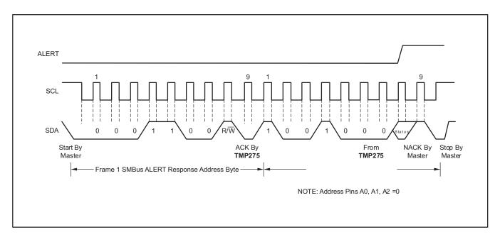
Figure 10. Timing Diagram for SMBus ALERT
