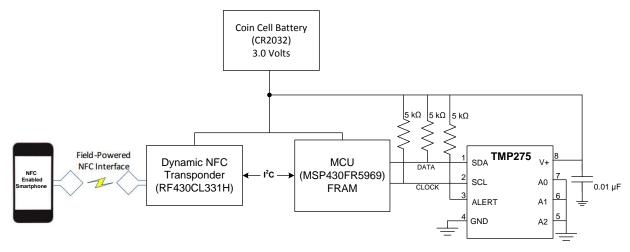
Figure 19. Temperature Data Logger
