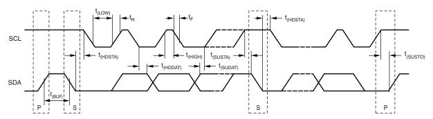
Figure 7. Two-Wire Timing Diagram
