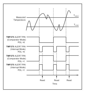
Figure 15. Output Transfer Function Diagrams
