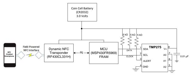
Figure 19. Temperature Data Logger
