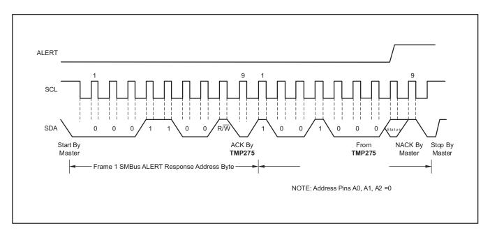
Figure 10. Timing Diagram for SMBus ALERT
