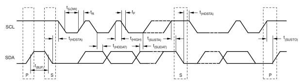
Figure 7. Two-Wire Timing Diagram
