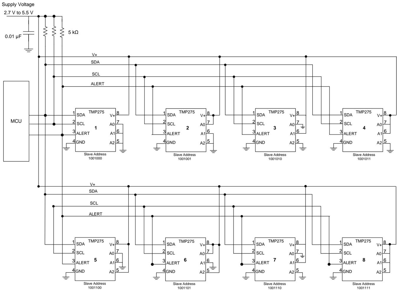
Figure 18. Connecting Multiple Devices on a Single Bus
