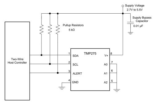
Figure 16. Typical Connections of the TMP275 Schematic
