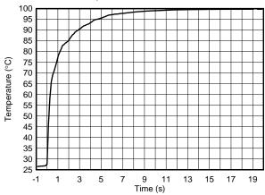
Figure 17. Temperature Step Response
