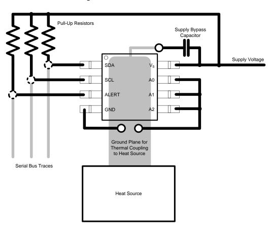
Figure 20. TMP275 Layout Example
