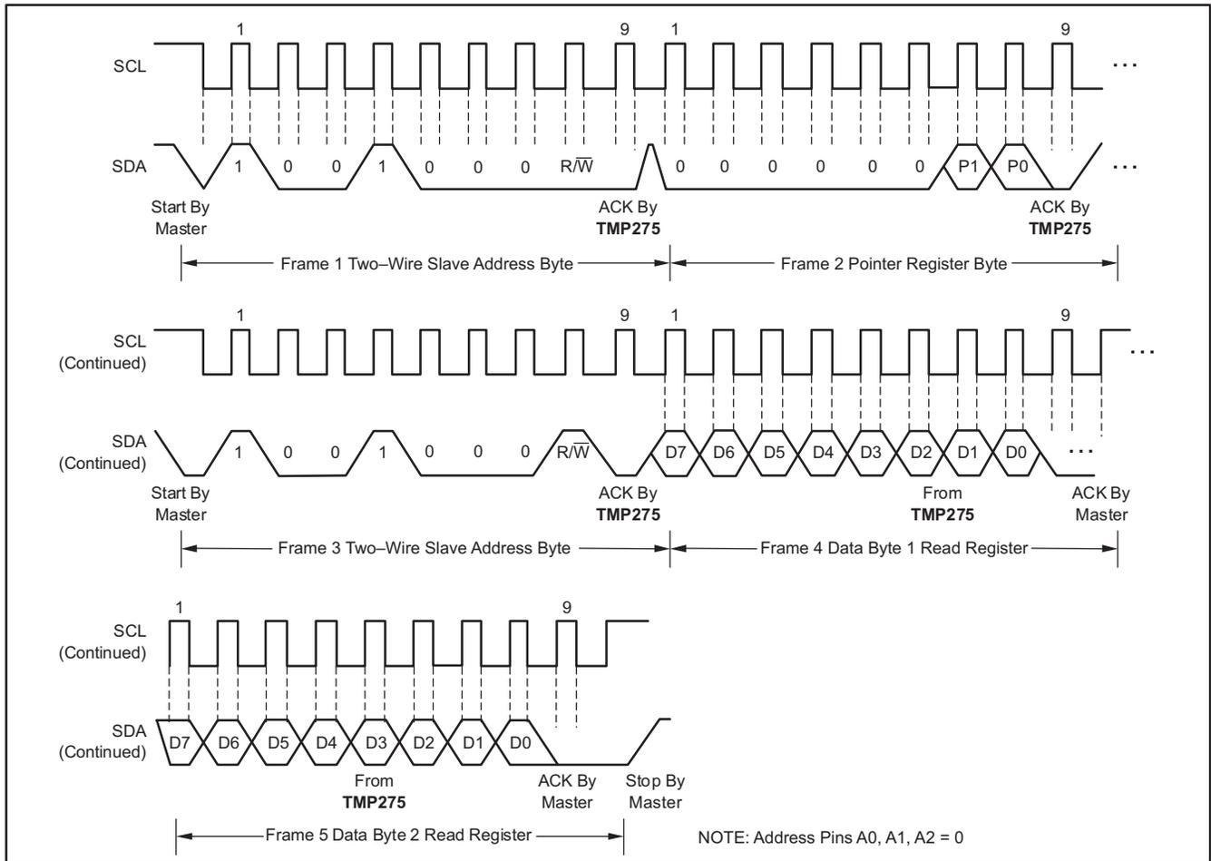
Figure 9. Two-Wire Timing Diagram for Read Word Format
