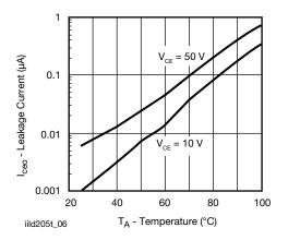
Fig. 10 - Collector Current vs. Ambient Temperature
