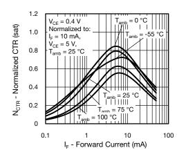
Fig. 7 - Normalized CTR (saturated) vs. Forward Current
