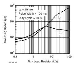
Fig. 9 - Switching Speed vs. Load Resistor
