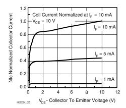
Fig. 5 - Collector Emitter Current vs.  $V_{\mbox{\scriptsize CE}}$
