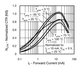
Fig. 6 - Normalized CTR (non-saturated) vs. Forward Current
