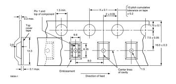
Fig. 12 - Tape Dimensions, 2000 Parts per Reel
