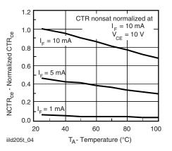
Fig. 8 - Current Transfer Ratio (normalized) vs. Ambient Temperature
