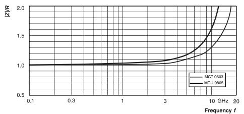
Relative impedance for 49.9  $\Omega$  chip resistor
