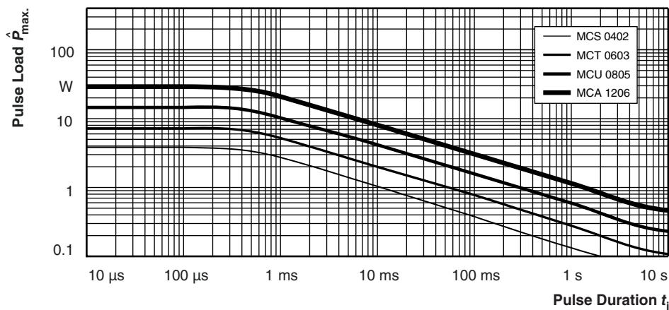
Maximum pulse load, single pulse; applicable if  $\bar{P} \rightarrow 0$  and  $n \leq 1000$  and  $\dot{U} \leq \dot{U}_{\text{max}}$ ;
