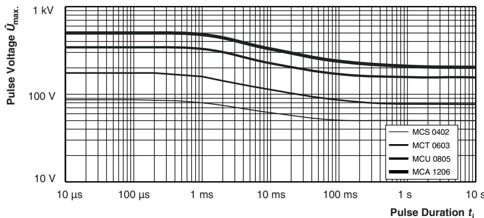
Maximum pulse voltage, single and continuous pulses; applicable if  $\hat{P} \leq \hat{P}_{\max}$ ;
