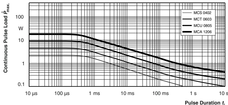
Maximum pulse load, continuous pulses; applicable if  $\bar{P} \leq P(\vartheta_{\text{amb}})$  and  $\dot{U} \leq \dot{U}_{\max}$ ;
