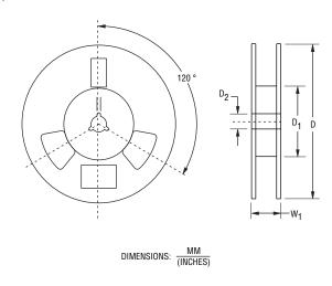
Devices are packed in accordance with EIA standard RS-481-A and specifications shown here.
