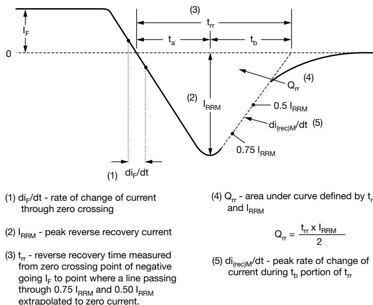
Fig. 9 - Reverse Recovery Waveform and Definitions
