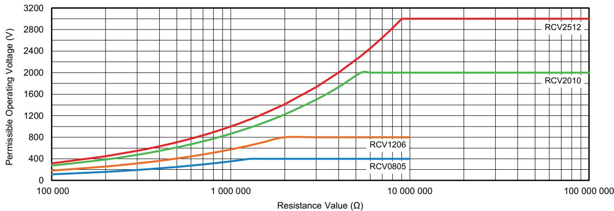
The permissible operating voltage  $U_{max}$  equals the rated voltage.
