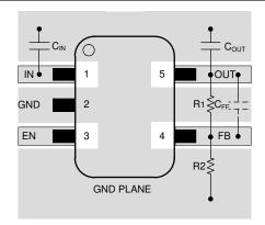
Figure 7-14. Layout Example for the DBV Package Adjustable Version
