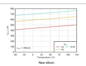
Figure 5-14. Ground Pin Current vs Temperature
