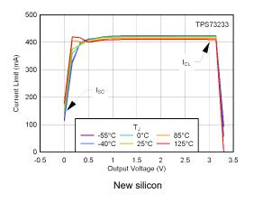
Figure 5-18. Current Limit vs V<sub>OUT</sub> (Foldback)
