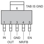
Figure 4-3. DCQ Package, 6-Pin SOT-223 (Top View)
