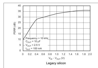
Figure 5-25. PSRR (Ripple Rejection) vs (V<sub>IN</sub> - V<sub>OUT</sub>)
