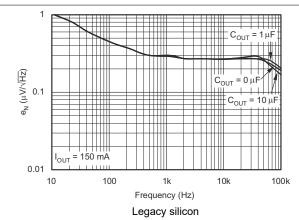
Figure 5-27. Noise Spectral Density  $C_{NR} = 0\mu F$
