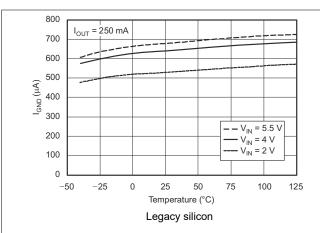
Figure 5-13. Ground Pin Current vs Temperature
