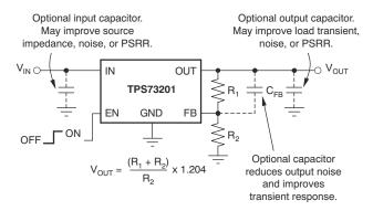
Figure 7-2. Typical Application Circuit for Adjustable-Voltage Version
