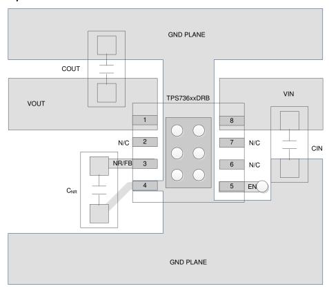
Figure 7-11. Fixed Output Voltage Option Layout (DRB Package)
