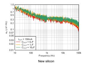
Figure 5-28. Noise Spectral Density  $C_{NR} = 0\mu F$
