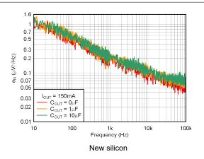
Figure 5-30. Noise Spectral Density  $C_{NR} = 0.01 \mu F$
