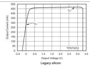
Figure 5-17. Current Limit vs V<sub>OUT</sub> (Foldback)
