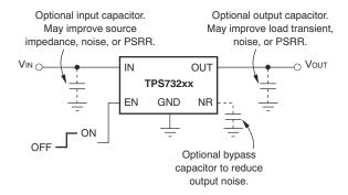
Figure 7-1. Typical Application Circuit for Fixed-Voltage Versions
