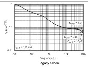
Figure 5-29. Noise Spectral Density  $C_{NR} = 0.01 \mu F$
