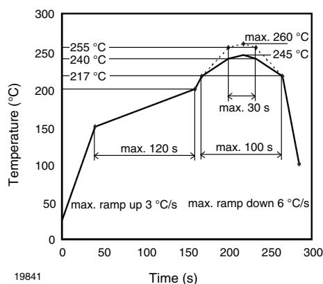
Fig. 7 - Lead (Pb)-free Reflow Solder Profile acc. J-STD-020D
