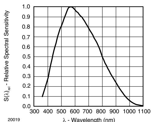
Fig. 5 - Relative Spectral Sensitivity vs. Wavelength
