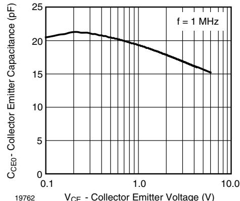
Fig. 4 - Collector Emitter Capacitance vs. Collector Emitter Voltage
