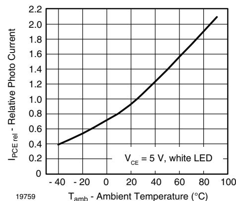
Fig. 2 - Relative Photo Current vs. Ambient Temperature
