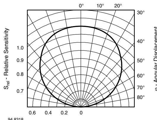
Fig. 6 - Relative Radiant Sensitivity vs. Angular Displacement
