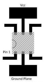
Figure 10-1. Recommended Layout Example
