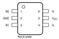
Figure 4-1. DBV Package, 6-Pin SOT-23 (Top View)
