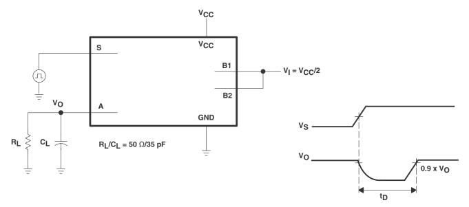
Figure 6-10. Break-Before-Make Internal Timing
