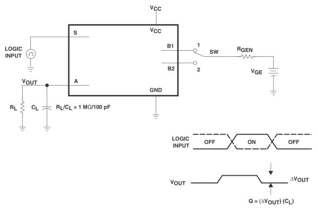
Figure 6-8. Charge-Injection Test
