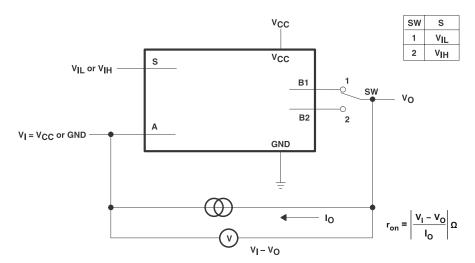
Figure 6-1. ON-State Resistance Test Circuit
