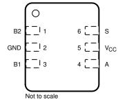
Figure 4-3. DRY Package, 6-Pin SON (Top View)
