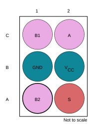
Figure 4-7. YZP Package, 6-Pin DSBGA (Bottom View)
