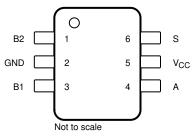
Figure 4-2. DCK Package, 6-Pin SC70 (Top View)
