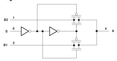
Figure 7-1. Logic Diagram (Positive Logic)
