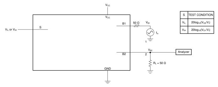
Figure 6-6. Crosstalk (Between Switches)
