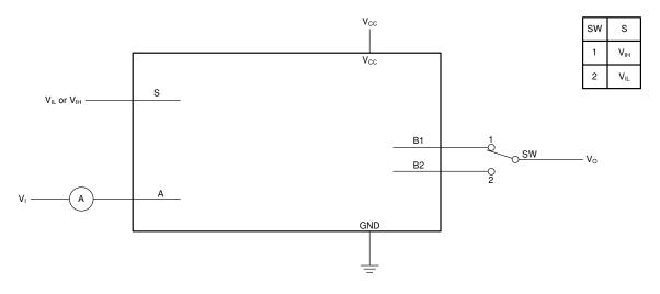
$\begin{aligned} & \text{Condition 1: } V_{I} = GND, \ V_{O} = V_{CC} \\ & \text{Condition 2: } V_{I} = V_{CC}, \ V_{O} = GND \end{aligned}$
