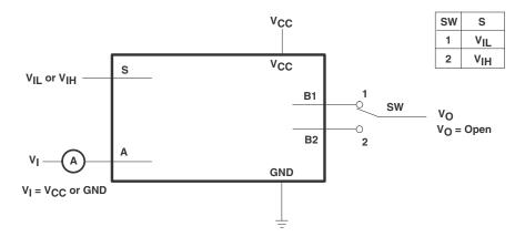
Figure 6-3. ON-State Switch Leakage-Current Test Circuit
