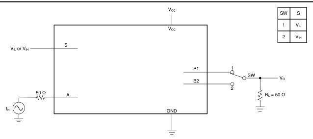
Figure 6-5. Frequency Response (Switch On)
