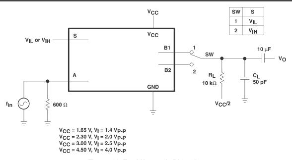
Figure 6-9. Total Harmonic Distortion
