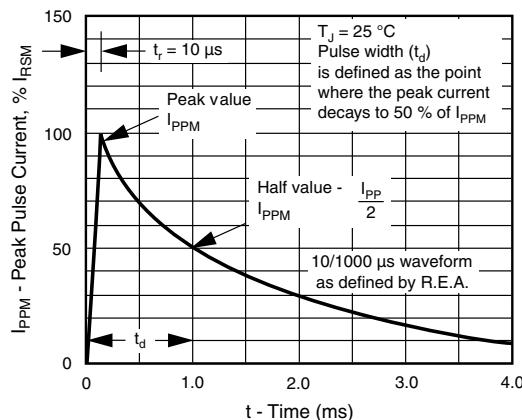
**Fig. 3 - Pulse Waveform**
