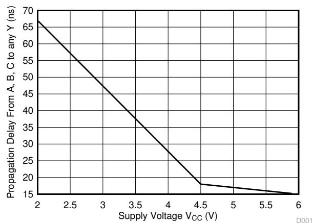
**Figure 6-1. Typical Propagation Delay vs Supply Voltage**
