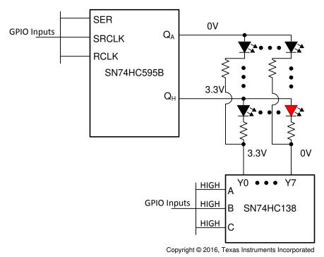
Figure 9-1. LED Matrix Driver Application
