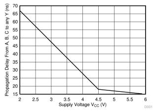
Figure 6-1. Typical Propagation Delay vs Supply Voltage
