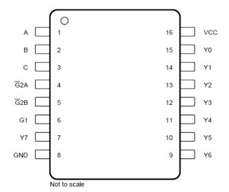
SOIC, SSOP, PDIP, SO, TSSOP, CDIP, or CFP Package 16-Pin D, DB, N, NS, PW, J or W Top View
