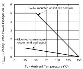
Fig. 5 - Power Dissipation Derating Curve
