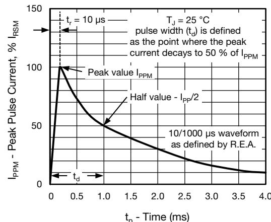
Fig. 3 - Pulse Waveform
