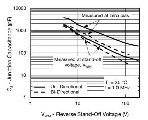
Fig. 4 - Typical Junction Capacitance
