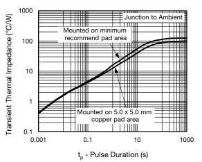
Fig. 6 - Typical Transient Thermal Impedance
