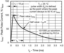
Fig. 3 - Pulse Waveform
