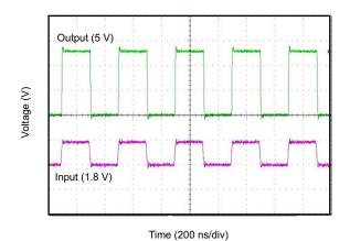
Figure 9-2. Translation Up (1.8 V to 5 V) at 2.5 MHz
