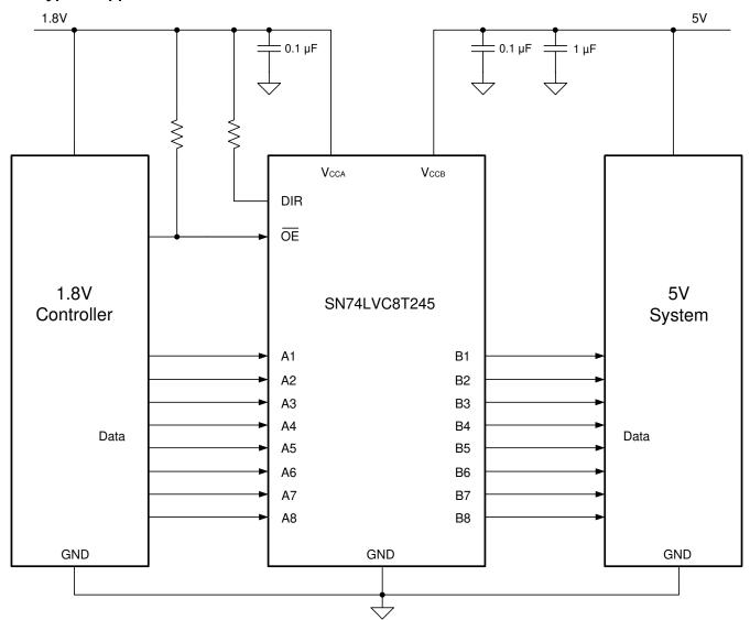
Figure 9-1. Typical Application Circuit
