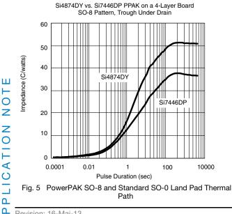
Because of the presence of the trough, this result suggests a minimum performance improvement of 10 °C/W by using a PowerPAK SO-8 in a standard SO-8 PC board mount.
