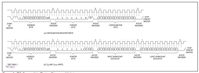
Figure 3. I<sup>2</sup>C-Compatible Timing Diagram (Write)
