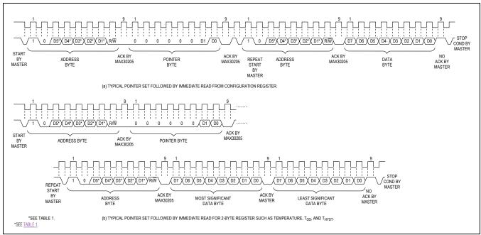
Figure 4. I<sup>2</sup>C-Compatible Timing Diagram (Read)
