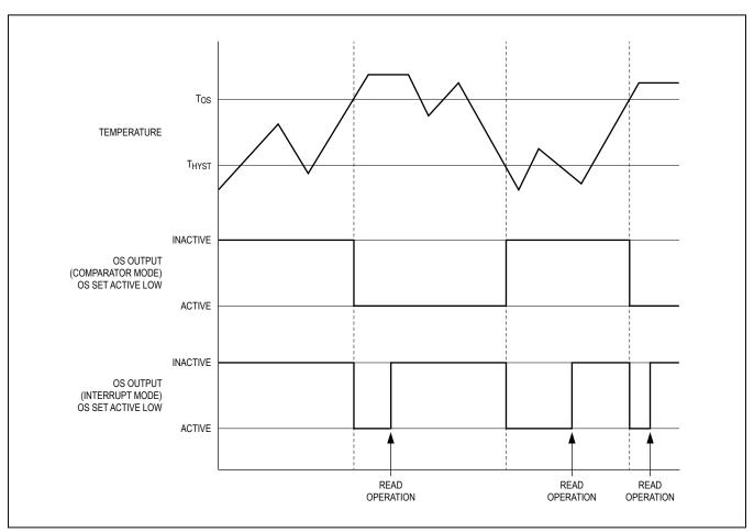
Figure 2. OS Output Temperature Response Diagram
