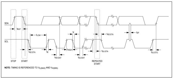
Figure 1. I<sup>2</sup>C Timing Diagram
