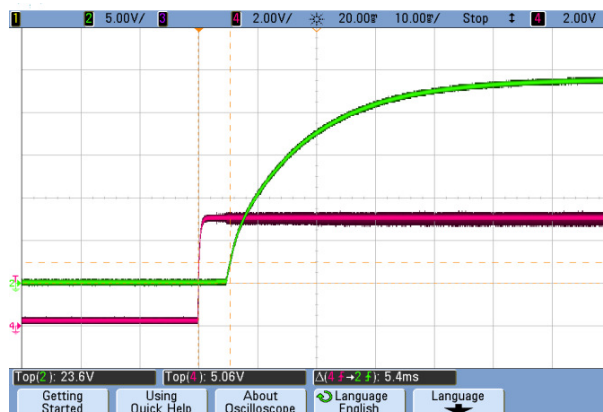
Transient Response (Vin = 12V, Vout = Nom, Iout = 50-75, Cloud = 1µF ceramic||10µF tantalum|| 100µF Ecap; Slew Rate = 1A/µs, Ta = 25°C)
