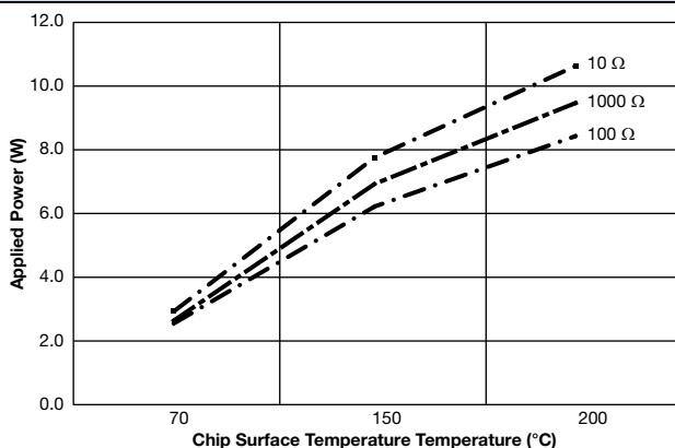
**PCNM2512 CHIP TEMP VS. APPLIED POWER**
