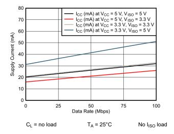
Figure 7-11. ISOW7841A-Q1 Supply Current vs **Data Rate**
