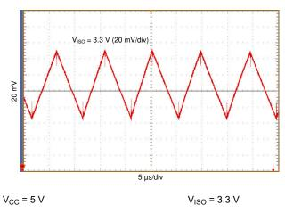
Figure 7-23. V<sub>ISO</sub> Ripple Voltage at 130 mA
