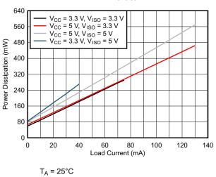
Figure 7-6. ISOW7841 Efficiency vs Load Current (I<sub>ISO</sub>)
