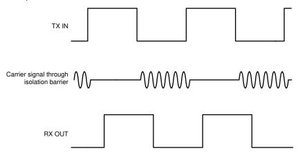
Figure 9-3. On-Off Keying (OOK) Based Modulation Scheme
