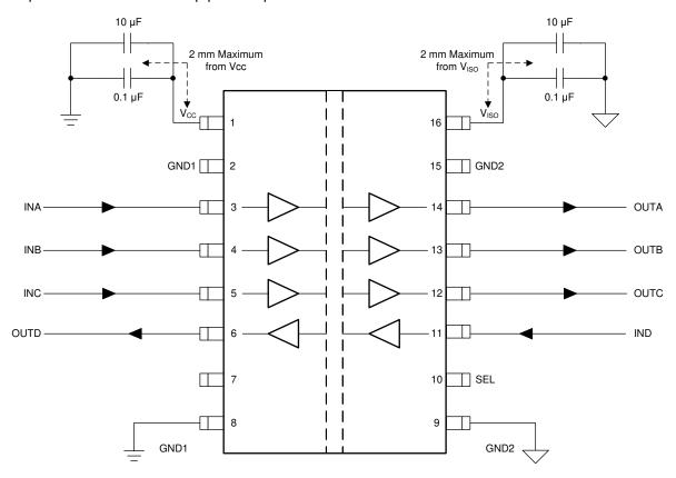
Figure 10-2. Typical ISOW7841A-Q1 Circuit Hook-Up
