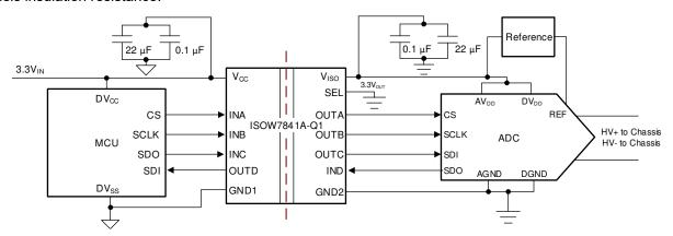
Figure 10-1. Isolated Power and SPI for Automotive BMS Insulation monitoring Application with ISOW7841A-Q1
