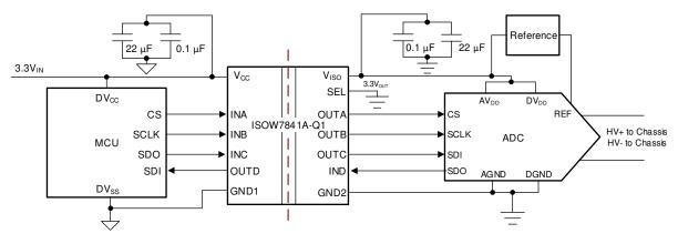
Figure 10-1. Isolated Power and SPI for Automotive BMS Insulation monitoring Application with ISOW7841A-Q1
