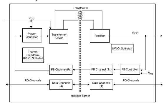
Figure 9-1. Block Diagram
