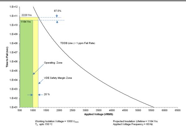
Figure 10-5. Insulation Lifetime Projection Data
