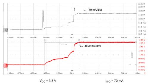
Input current spike is because of charging the input supply decoupling capacitor
