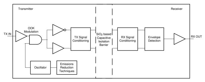
Figure 9-2. Conceptual Block Diagram of a Capacitive Data Channel
