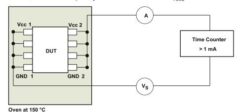
Figure 10-4. Test Setup for Insulation Lifetime Measurement
