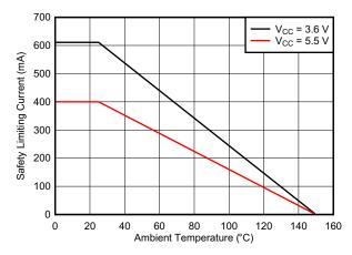
Figure 7-1. Thermal Derating Curve for Safety Limiting Current per VDE
