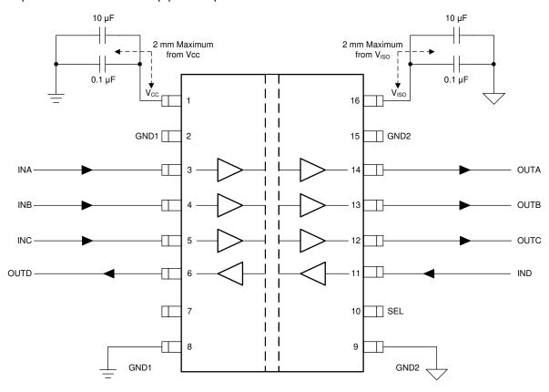
Figure 10-2. Typical ISOW7841A-Q1 Circuit Hook-Up
