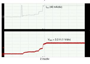
$V_{CC}$  = 5 V  $V_{ISO}$  = 3.3 V Input current spike is because of charging the input supply decoupling capacitor
