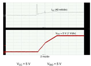
Input current spike is because of charging the input supply decoupling capacitor
