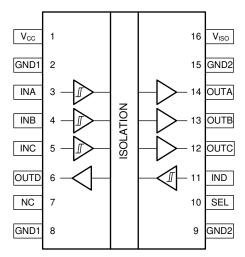
ISOW7841A-Q1 DWE Package. 16-Pin SOIC-WB. Top View.
