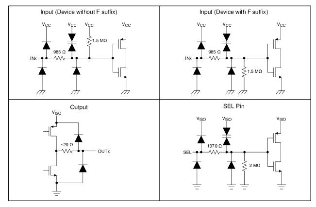
Figure 9-4. Device I/O Schematics
