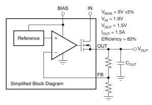
Figure 7-2. Typical Application of the TPS748 Using an Auxiliary Bias Rail
