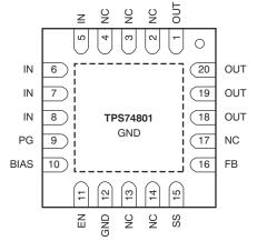
Figure 4-2. RGW Package, 20-Pin VQFN (Top View)
