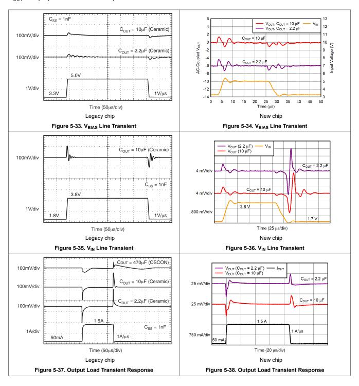
at  $T_J$  = 25°C,  $V_{IN}$  =  $V_{OUT(nom)}$  + 0.3 V,  $V_{BIAS}$  = 5 V,  $I_{OUT}$  = 1 A,  $V_{EN}$  =  $V_{IN}$  = 1.8 V,  $V_{OUT}$  = 1.5 V,  $C_{IN}$  = 1  $\mu$ F,  $C_{BIAS}$  = 4.7  $\mu$ F, and  $C_{OUT}$  = 10  $\mu$ F (unless otherwise noted)
