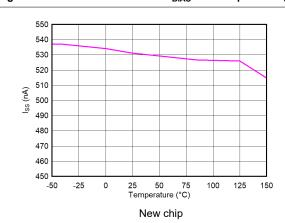
Figure 5-28. Soft-Start Charging Current (I<sub>SS</sub>) vs Temperature  $(T_J)$
