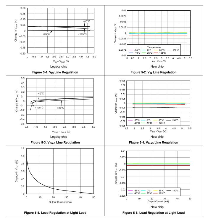
at  $T_J$  = 25°C,  $V_{IN}$  =  $V_{OUT(nom)}$  + 0.3 V,  $V_{BIAS}$  = 5 V,  $I_{OUT}$  = 50 mA,  $V_{EN}$  =  $V_{IN}$ ,  $C_{IN}$  = 1  $\mu$ F,  $C_{BIAS}$  = 4.7  $\mu$ F, and  $C_{OUT}$  = 10  $\mu$ F (unless otherwise noted)
