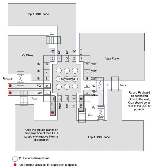
Figure 7-16. Layout Example (RGW Package)
