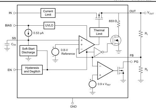
Figure 6-2. New Chip Functional Block Diagram
