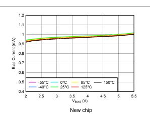
Figure 5-26. BIAS Pin Current vs V<sub>BIAS</sub> and Temperature (T<sub>J</sub>)
