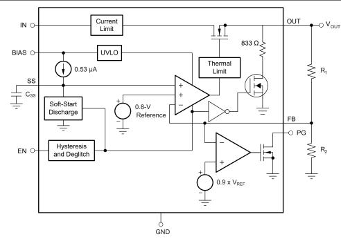
Figure 6-2. New Chip Functional Block Diagram
