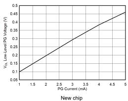
Figure 5-30. Low-Level PG Voltage vs Current
