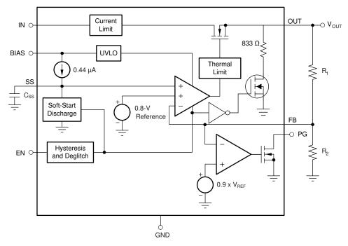
Figure 6-1. Legacy Chip Functional Block Diagram
