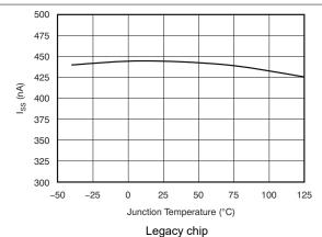
Figure 5-27. Soft-Start Charging Current (I<sub>SS</sub>) vs Temperature  $(T_J)$
