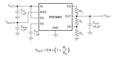
Figure 7-1. Typical Application Circuit for the TPS748 (Adjustable)
