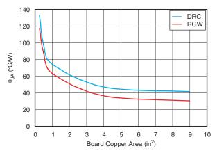
$R_{\theta JA}$  value at board size of 9 in² (that is, 3 in  $\times$  3i n) is a JEDEC standard.
