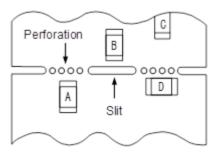
(3) Mounting components near screw holes
