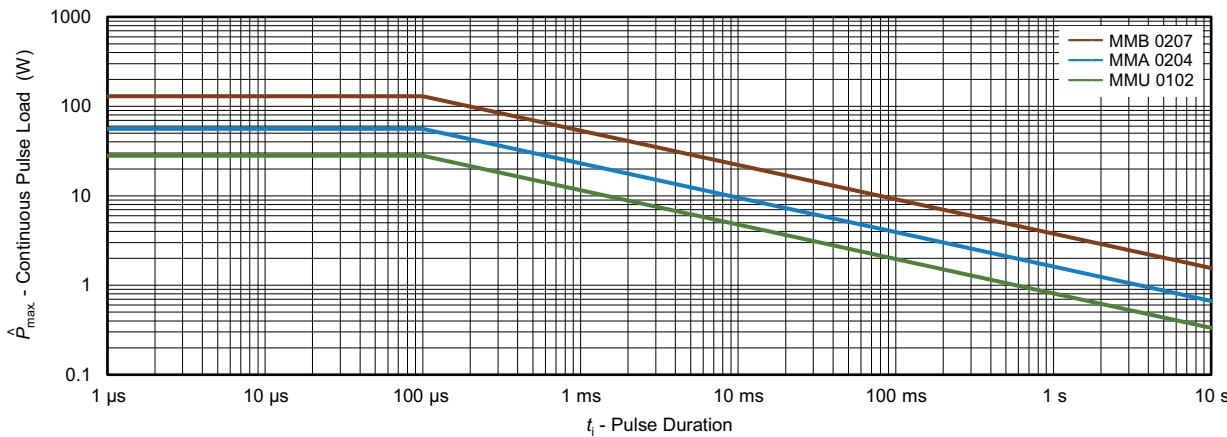
Maximum pulse load, continuous pulse; applicable if  $\bar{P} \leq P(\vartheta_{\text{amb}})$  and  $\hat{U} \leq \hat{U}_{\max}$ ;
