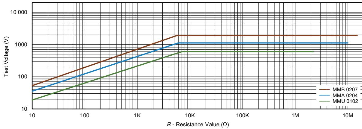
Pulse load rating in accordance with EN 60115-1 clause 8.2; 10 μs / 700 μs;
