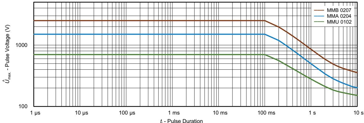
Maximum pulse voltage, single and continuous pulses; applicable if  $\hat{P} \leq \hat{P}_{\max}$ ;
