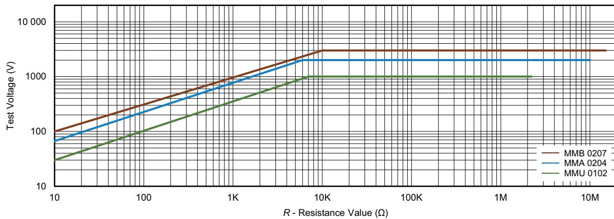
Pulse load rating in accordance with EN 60115-1 clause 8.2; 1.2 μs / 50 μs;
