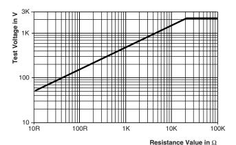
Pulse load rating in accordance with IEC 60115-1, 4.27; 10  $\mu$ s / 700  $\mu$ s; 10 pulses at 1 minute intervals; for permissible resistance change  $\pm$  (0.5 % R + 0.05  $\Omega$ )
