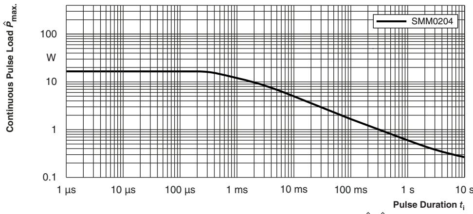
Maximum pulse load, continuous pulse; applicable if  $\bar{P} \leq P (9_{\text{amb}})$  and  $\hat{U} \leq \hat{U}_{\max}$ ;
