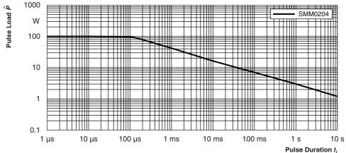
Maximum pulse load, single pulse; applicable if  $\bar{P}$   $\rightarrow$  0 and n  $\leq$  1000 and  $\hat{U} \leq \hat{U}_{\text{max}}$ ; for permissible resistance change  $\pm$  (0.5 % R + 0.01  $\Omega$ )
