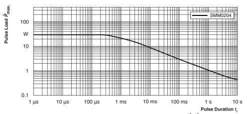
Maximum pulse load, single pulse; applicable if  $\vec{P} \longrightarrow 0$  and  $n \le 1000$  and  $\hat{U} \le \hat{U}_{\max}$ ; for permissible resistance change  $\pm$  (0.5 % R + 0.01  $\Omega$ )
