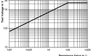
Pulse load rating in accordance with IEC 60 115-1, 4.27; 1.2  $\mu s$  / 50  $\mu s$ ; 5 pulses at 12 s intervals; for permissible resistance change  $\pm$  (0.5 % R + 0.05  $\Omega$ ) 1.2 / 50 Pulse
