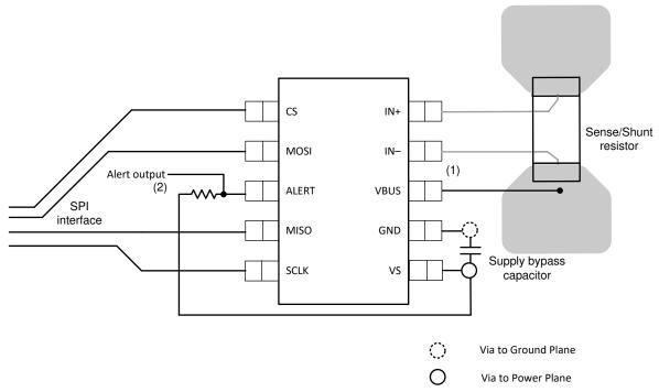
(1) Connect the VBUS pin to the voltage powering the load for load power calculations..
