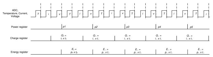
Figure 7-2. Power, Energy and Charge Calculation Scheme
