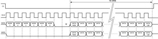
Figure 7-8. SPI Write Frame
