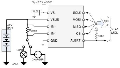
Figure 8-2. INA229-Q1 High-Side Sensing Application Diagram
