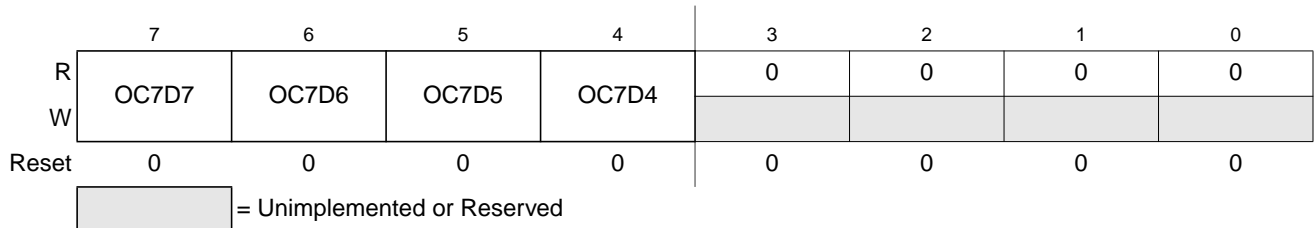
Figure 13-6. Output Compare 7 Data Register (OC7D)
