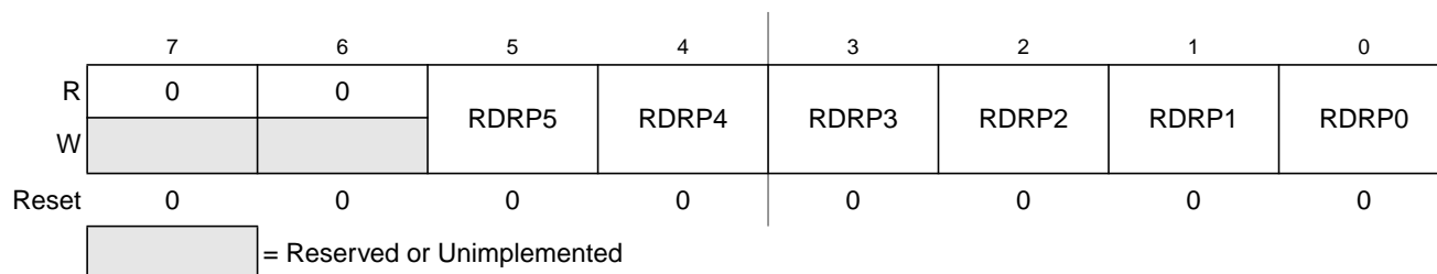
Figure 3-20. Port P Reduced Drive Register (RDRP)
