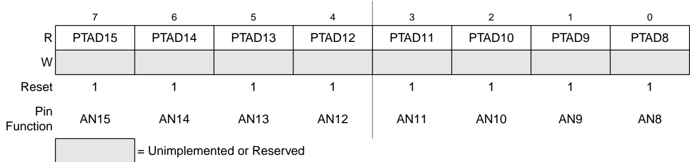
Figure 6-16. Port Data Register 0 (PORTAD0)
