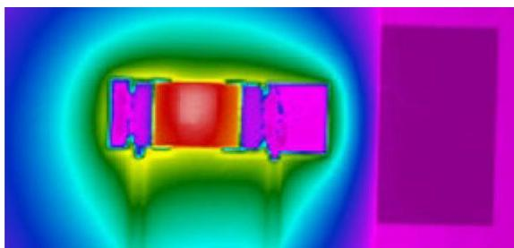
Ceramic Resistor Chip Without Thermal Jumper (149.8 °C)
