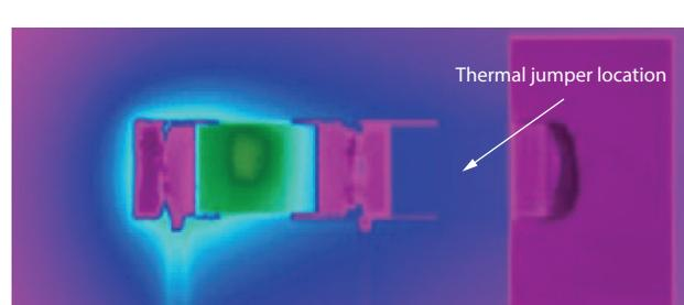
Ceramic Chip Resistor With Thermal Jumper (95.5 °C)
