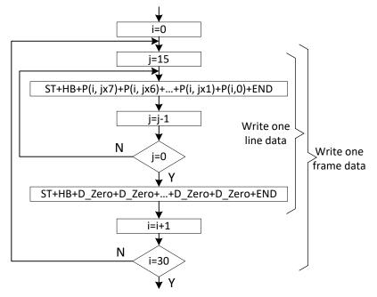
Figure 9-4. Data Write Flow
