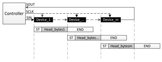
Figure 8-18. Chip Index Write Command
