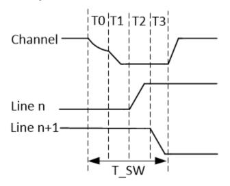
Figure 8-7. Line Transitioning Sequence
