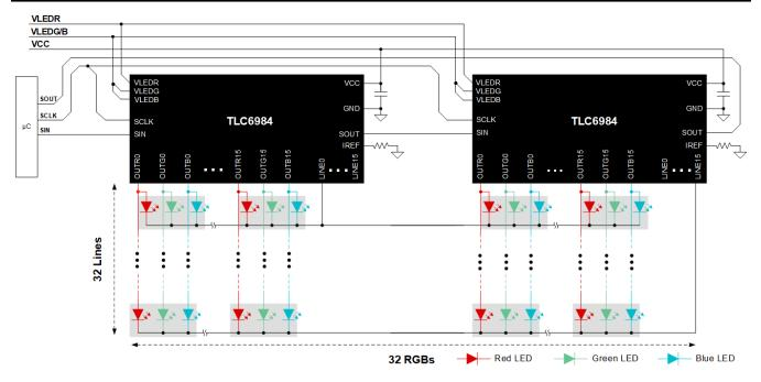
Figure 9-1. TLC6984 With Dual Devices Stackable Connection
