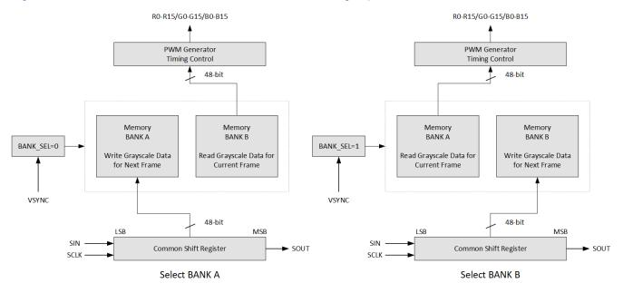
Figure 8-26. Bank Selection Exchange Operation
