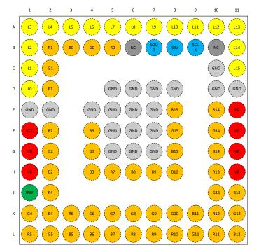
Figure 6-2. TLC6984 ZXL Package 96-Pin BGA Top View
