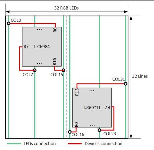
Figure 11-4. Channel Routing Suggestion With Channel Order Sequence
