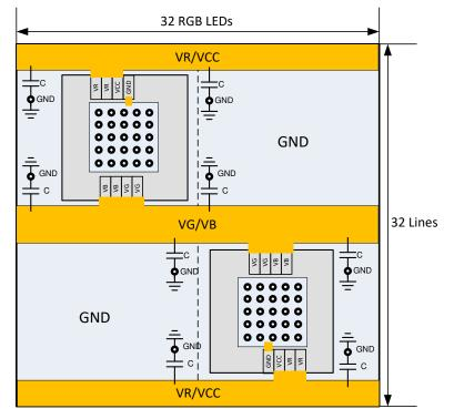
Figure 11-1. Power Rails Routing Suggestion
