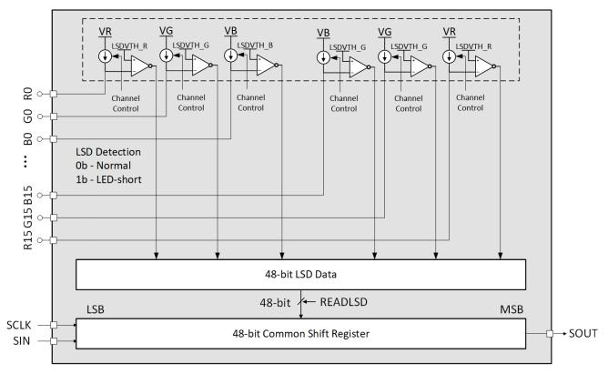
Figure 8-12 shows the equivalent circuit of LED short detection.
