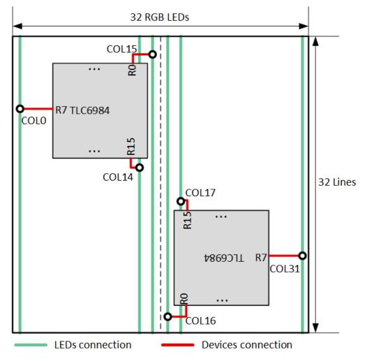
Figure 11-3. Channel Routing Suggestion With Shortest Wire
