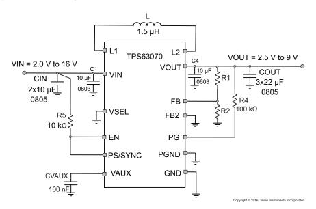
Figure 10. Typical Application For Adjustable Version
