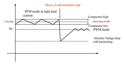
Figure 9. Dynamic Voltage Positioning
