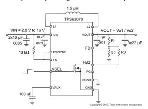
Figure 8. Typical Application using VSEL
