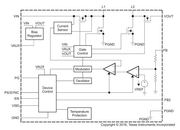
Figure 6. Functional Block Diagram
