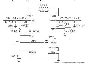
Figure 8. Typical Application using VSEL
