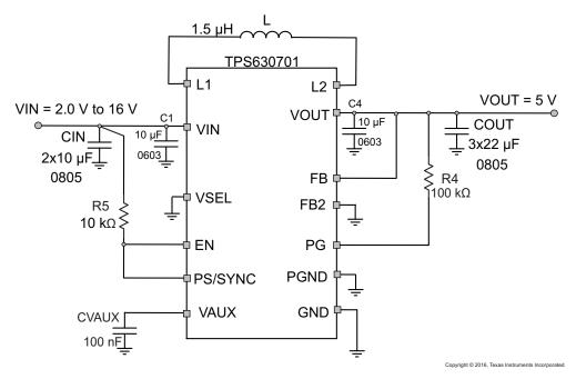
Figure 37. Typical Application For Fixed Voltage Version With Minimum External Part Count And Minimum Soft Start Time
