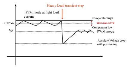
Figure 9. Dynamic Voltage Positioning
