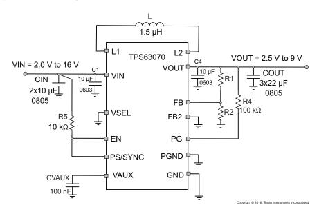
Figure 10. Typical Application For Adjustable Version
