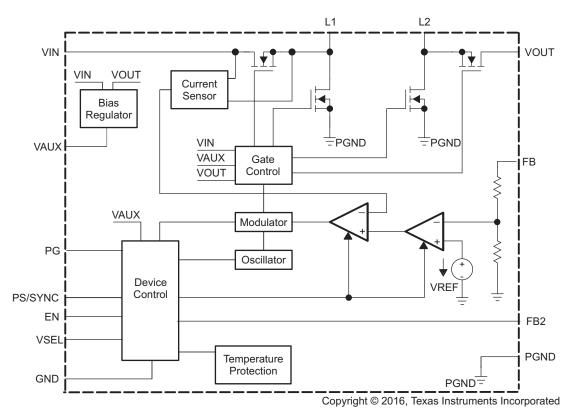
Figure 6. Functional Block Diagram
