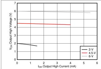
Figure 5-1. Typical output voltage in the high state  $(V_{OH})$
