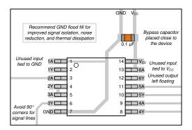
Figure 8-3. Example layout for the SN74HC14
