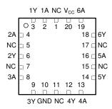
Figure 4-2. FK Package 20-Pin LCCC Top View
