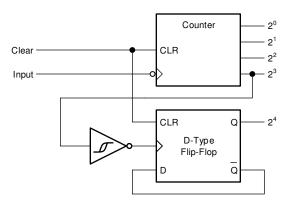
Figure 8-1. Typical application schematic
