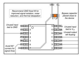
Figure 8-3. Example layout for the SN74HC14
