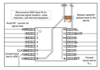
Figure 8-3. Example Layout for the SNx4HC166
