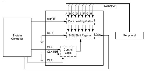
Figure 8-1. Typical Application Block Diagram
