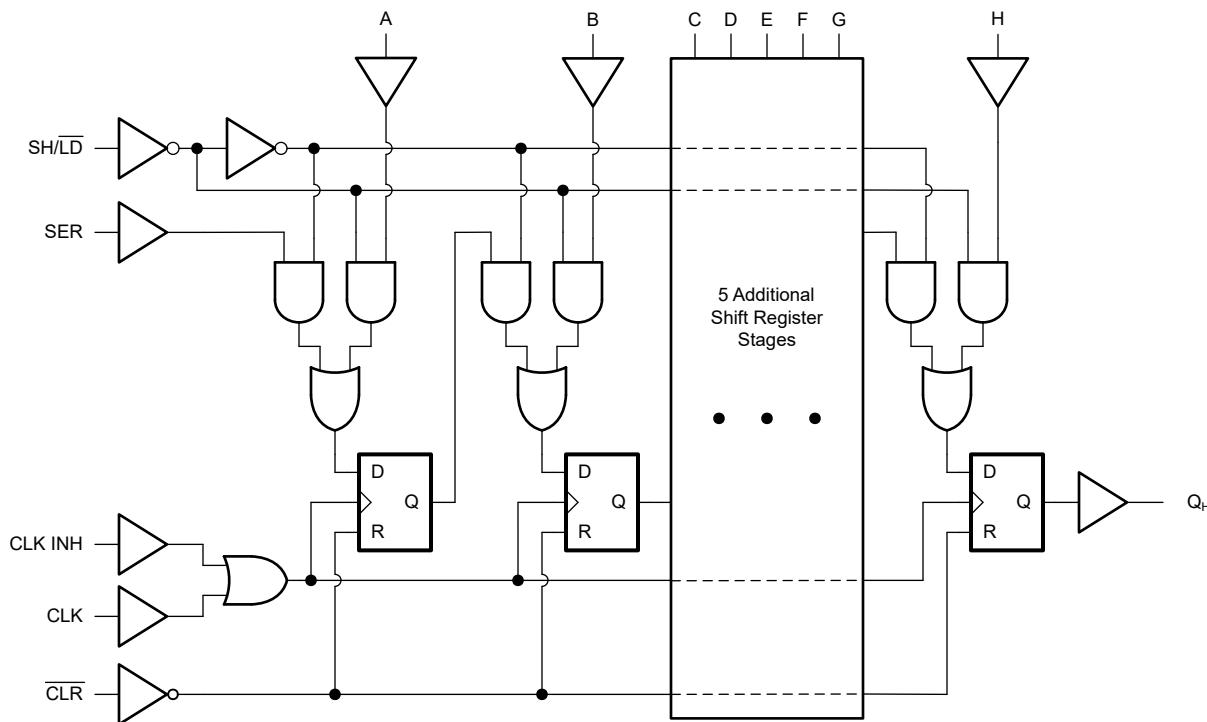
Figure 7-1. Logic Diagram (Positive Logic) for SNx4HC166
