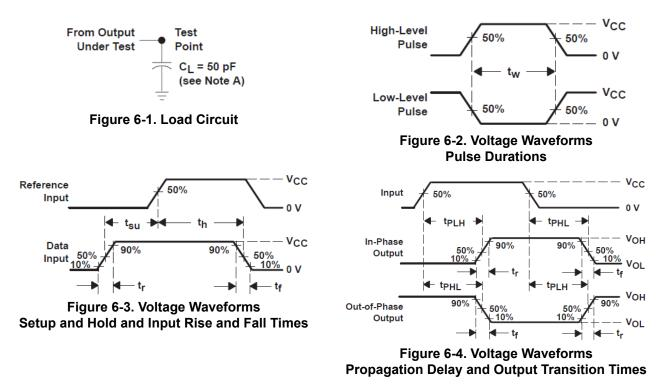
A. C<sub>L</sub> includes probe and jig capacitance.
