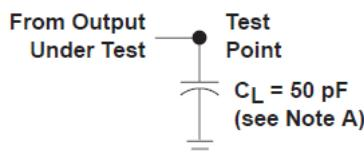
Figure 6-1. Load Circuit
