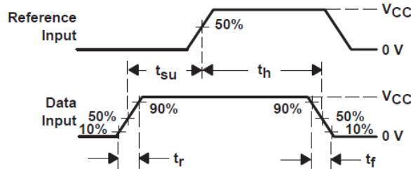
Figure 6-3. Voltage Waveforms
