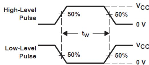
Figure 6-2. Voltage Waveforms
