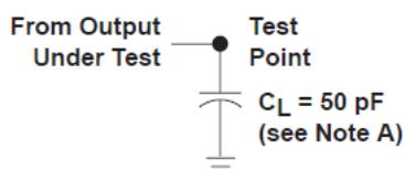
Figure 7-1. Load Circuit
