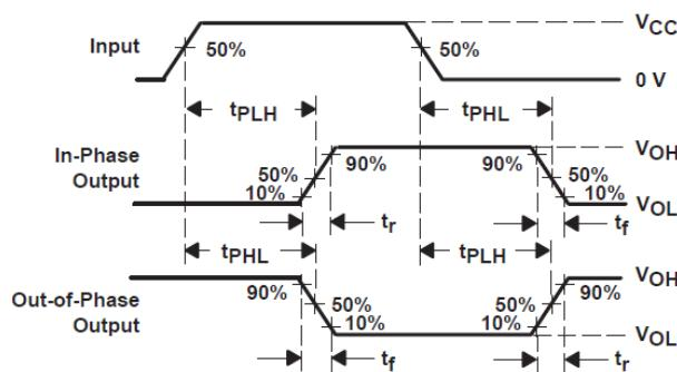
Figure 7-4. Voltage Waveforms
