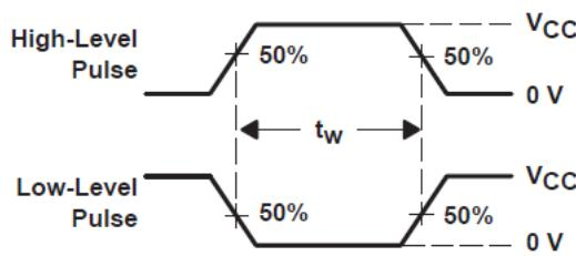
Figure 7-2. Voltage Waveforms
