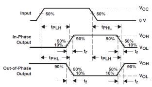
Figure 7-4. Voltage Waveforms
