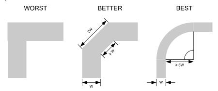
Figure 7-3. Example trace corners for improved signal integrity
