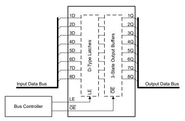
Figure 7-1. Typical Application Block Diagram
