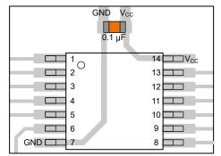
Figure 7-4. Example bypass capacitor placement for TSSOP and similar packages
