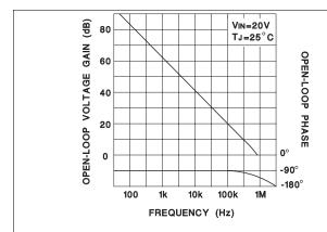
Figure 1. Error Amplifier Gain and Phase vs Frequency
