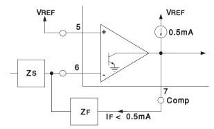
Error Amplifier can source up to 0.5mA.
