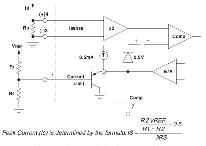
Figure 8. Pulse by Pulse Current Limiting
