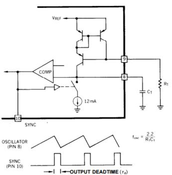
Figure 4. Oscillator Circuit
