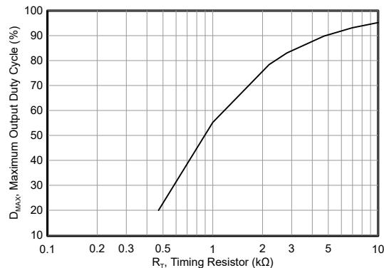
**Figure 5-9. Maximum Output Duty Cycle vs Timing Resistor**
