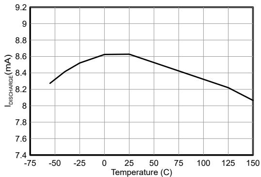
**Figure 5-4. Oscillator Discharge Current vs Temperature**
