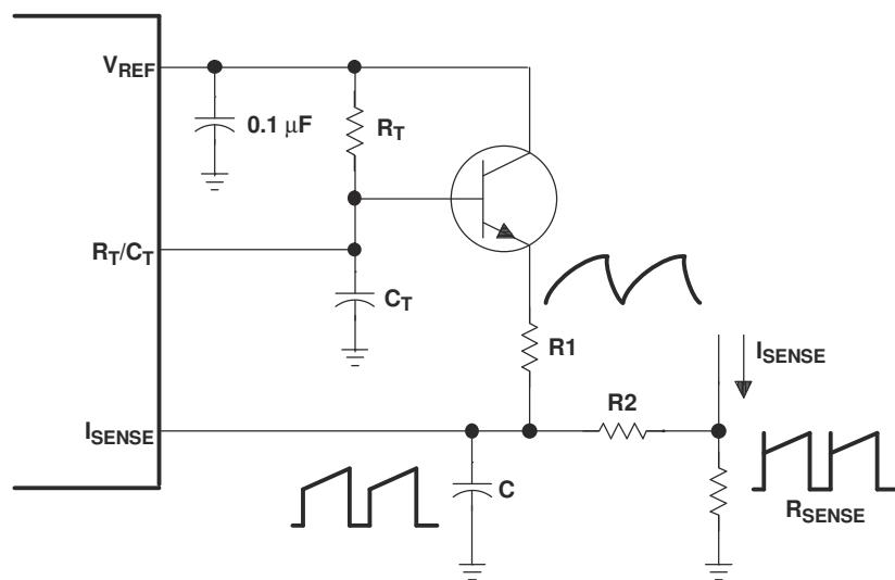
**Figure 7-5. Slope Compensation**
