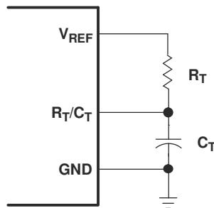
**Figure 7-3. Oscillator Section**
