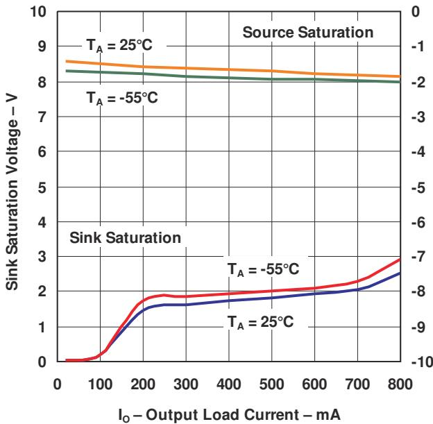
**Figure 5-8. Output Saturation Voltage vs Load Current**
