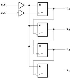
Logic Diagram, Each Counter (Positive Logic)
