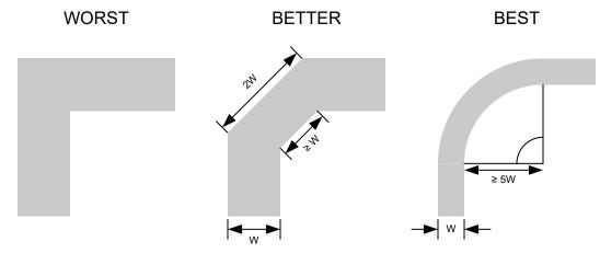
Figure 7-1. Example Trace Corners for Improved Signal Integrity
