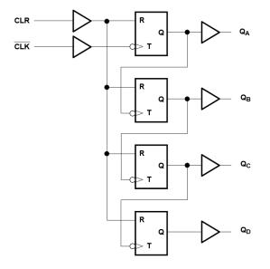
Figure 6-1. Logic Diagram, Each Counter (Positive Logic)
