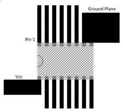
Figure 8-2. Layout Example Schematic
