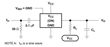
Figure 6-6. Frequency Response (Switch On)
