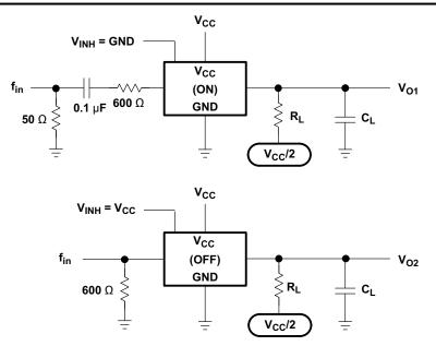
Figure 6-7. Crosstalk Between Any Two Switches
