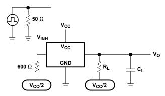
Figure 6-8. Crosstalk Between Control Input and Switch Output
