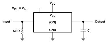
Figure 6-4. Propagation Delay Time, Signal Input to Signal Output
