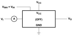
$\begin{array}{l} \text{Condition 1: V}_{\text{I}} = 0, \, \text{V}_{\text{O}} = \text{V}_{\text{CC}} \\ \text{Condition 2: V}_{\text{I}} = \text{V}_{\text{CC}}, \, \text{V}_{\text{O}} = 0 \\ \end{array}$
