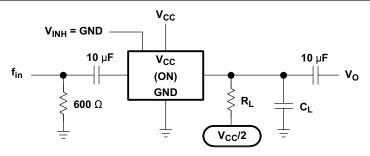
Figure 6-10. Sine-Wave Distortion
