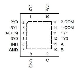
Figure 4-2. SN74LV4053A RGY, 16-Pin VQFN (Top View)
