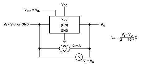
Figure 6-1. On-State Resistance Test Circuit
