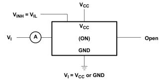
Figure 6-3. On-State Switch Leakage-Current Test Circuit
