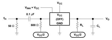
Figure 6-9. Feedthrough Attenuation (Switch Off)
