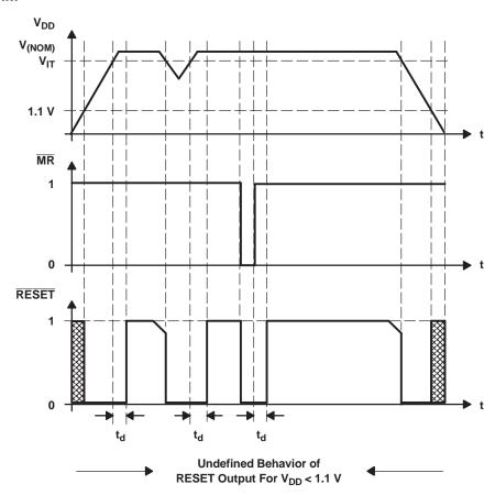
NOTE:  $\overline{\text{RESET}}$  should not be forced high during the power-up sequence (until  $V_{DD} > 1.1 \text{ V}$ ).
